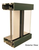
Fully pressure equalized with a rain screen gasket to eliminate the exterior seal between glazed units, PG 123<sup>TM</sup> Framing is fully tested to appropriate AAMA, ASTM and CAN/CSA A-440 standards for air, water and structural performance.
